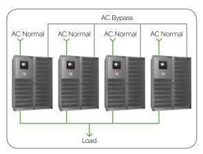
Distributed parallel connection for increased power and redundancy
