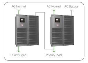
Live standby redundancy
