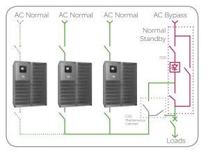
Parallel connection for increased power with a centralized static switch (CSS) unit and up to 8 UPS units, including the optional Centralized Static Switch Bypass which enables maintenance of the CSS while continuing to support the load
